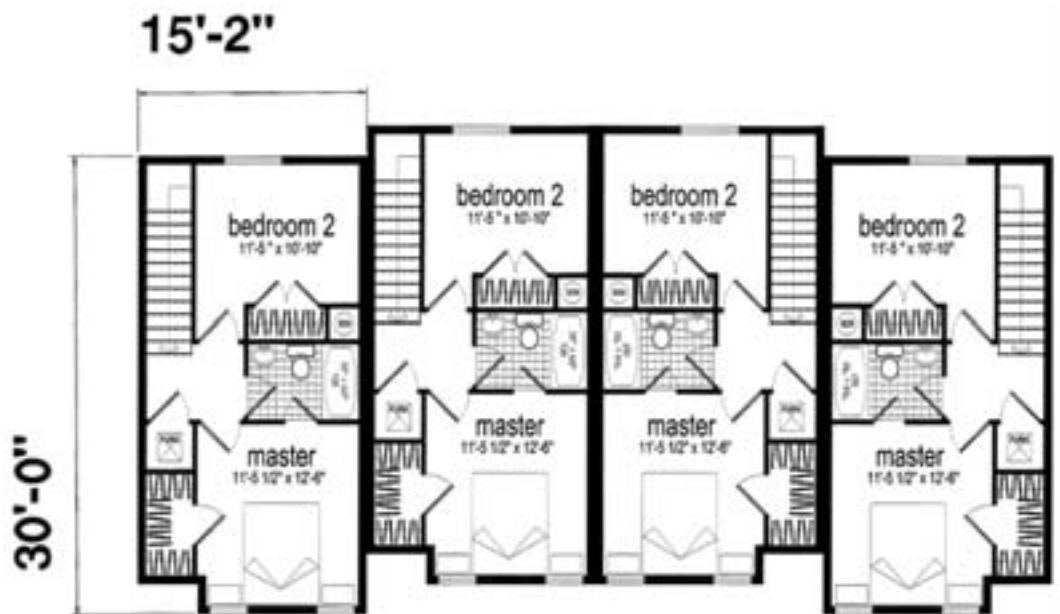
FIGURE 6 Second floor plan of two-story four-plex, Upton Street Community
