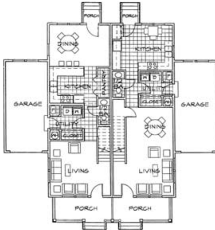
FIGURE 32 First-floor plan of HUD-code duplex, Noji Gardens
